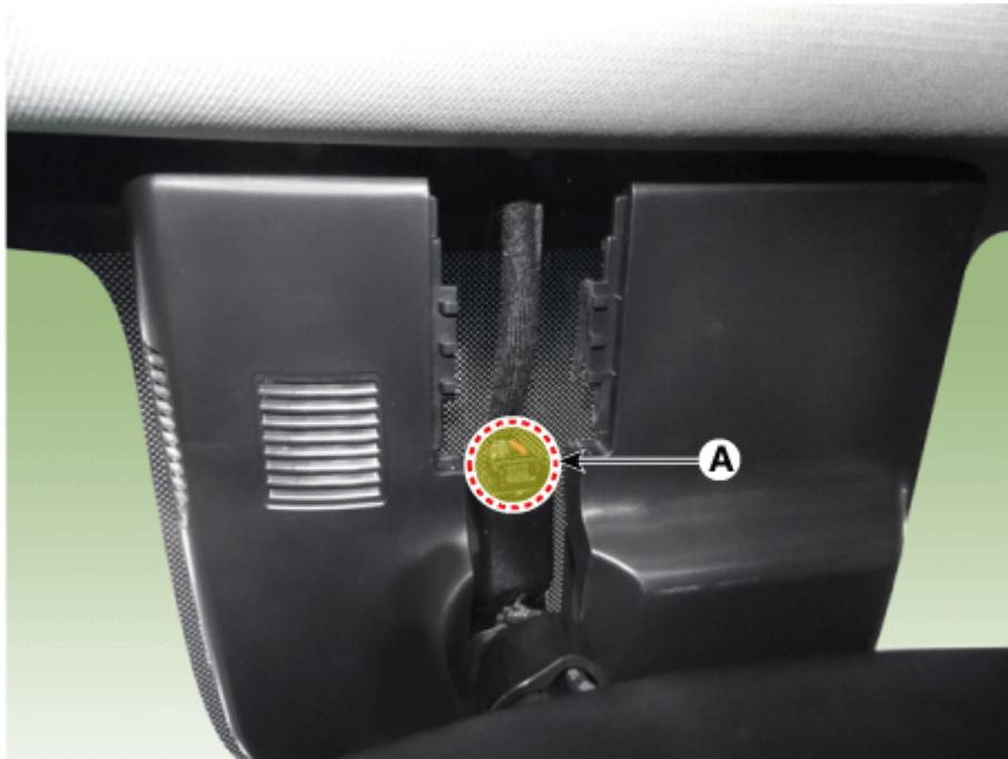
3. Push the ECM mirror base down to remove the ECM mirror assembly (A).
